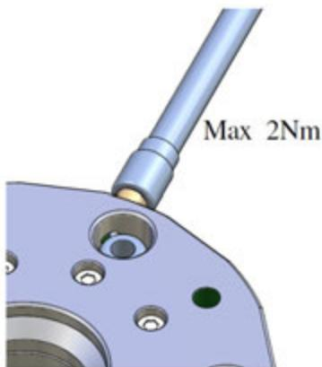
After assembly it is possible to use the screw set in order to eliminate any play between the two sides with "zero tolerance"
